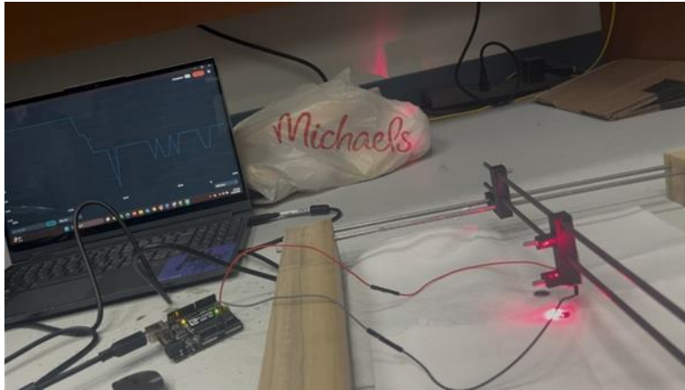
Figure 50: The carriage was just moved onto a black spot on cotton fabric. Photodiode readings on the graph on the left show significantly reduced back-reflections.
