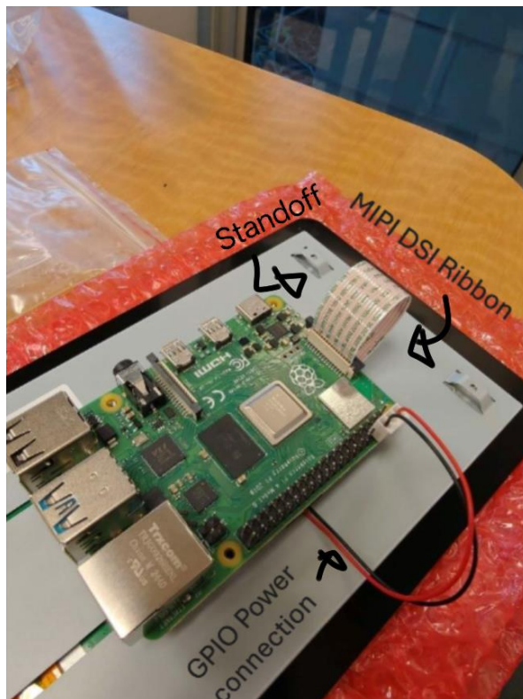
Figure 41: Touch Display 2 to Raspberry Pi 4B Connection
