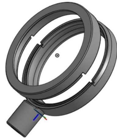
Figure 27: Snap Lens Mount for LB1945-A
